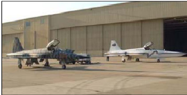
Unmodified F-5E and modified Shaped Sonic Boom Demonstrator (SSBD) aircraft. [DARPA /NASA /Northrop-Grumman]
