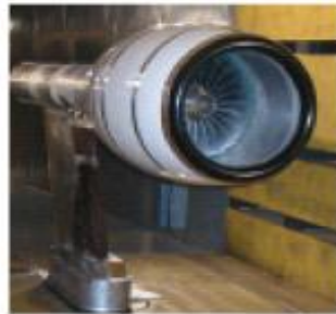
Fan Noise Reduction (Forward swept fan, porous stators, variable area fan nozzle)
