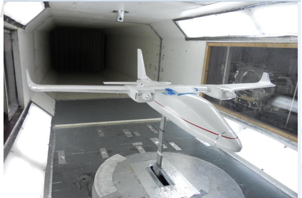
Wind Tunnel Tests were performed on a scale model of the aircraft, which confirmed and validated the CFD and preliminary aerodynamic analysis.
