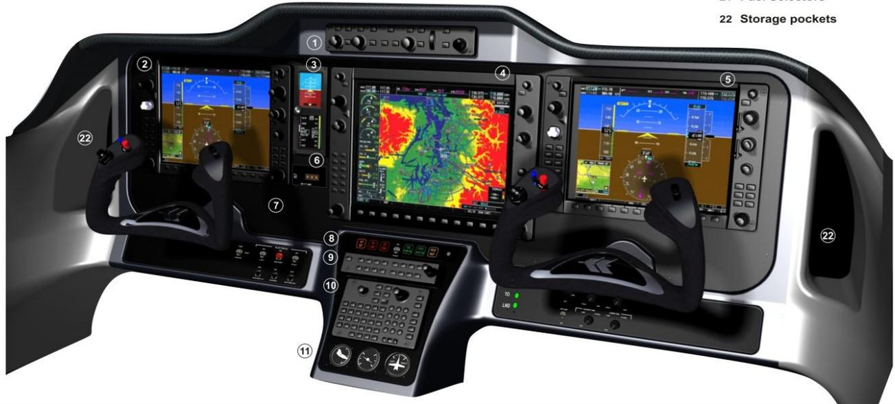
The KN-63 DME information is integrated within the display and offers Nav1/Nav2 switching. Crew alerts are displayed on the PFD. The automatic flight control system (AFCS) incorporates a GFC-700 three-axis autopilot with pitch trim.
