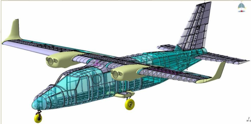
P2012 fuselage is composed by aluminium formed sheet metal frames, beams, stringers and panels coupled by solid rivets or, where necessary, by bolts. Some major items, as undercarriage beams, wing and tail surface attachments, are machined.
