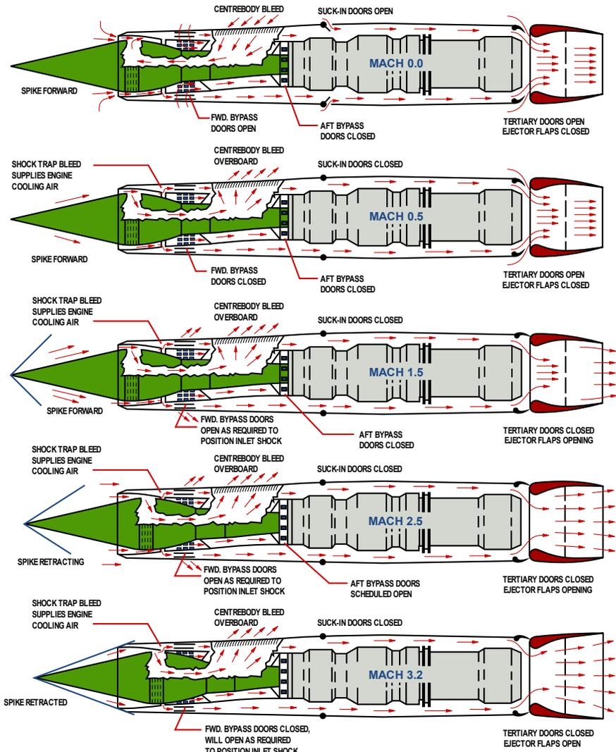
Operation of the air inlet and nozzle showing air flow through the nacelle
