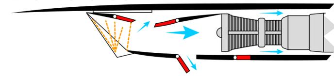
Need for mechanical actuators and control systems for intake movable ramps and/or deflectors and nozzle petals
