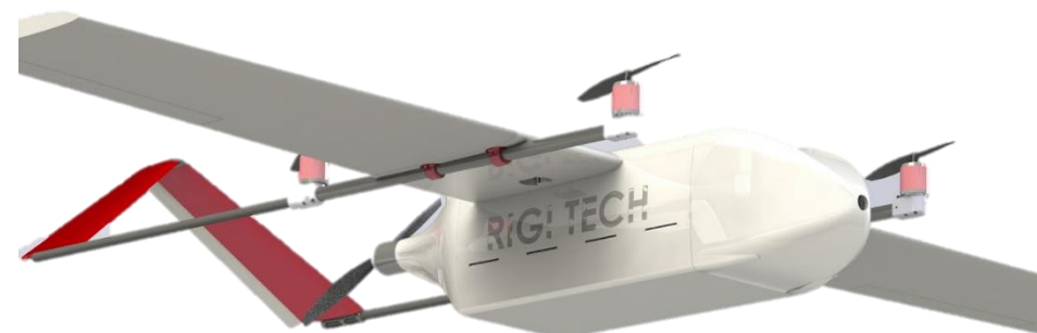
Octacopter ID8HSE (10 kg payload)
