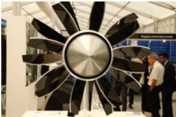
Figure 9.3 – Airbus concept aircraft with a noise shielded integration of an advanced CROR engine
