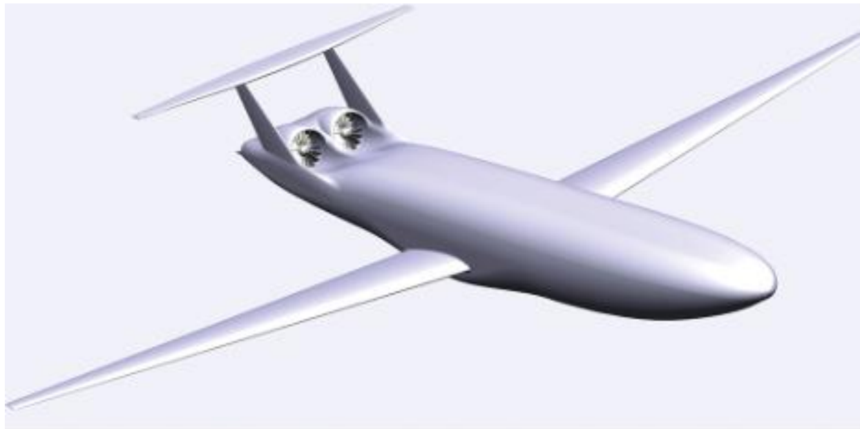
Clustered beneath the pi-tail of the NASA/MIT D8 design, the engine location presents certification and configuration challenges. Credit: NASA
