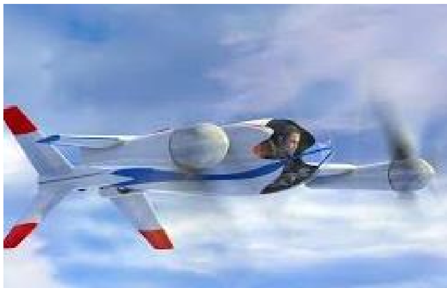
DISTRIBUTED ELECTRIC PROPULSION AIRCRAFT (NASA- TECNAM: Dr. Moore)
