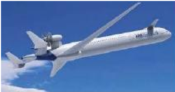
Figure 9.3 – Airbus concept aircraft with a noise shielded integration of an advanced CROR engine
