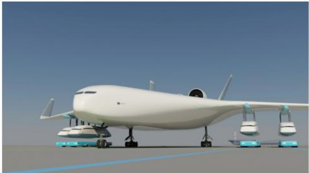
The Fantassy study looked at how aircraft could carry intermodal passenger pods between airports. Credit: Fantassy Project
