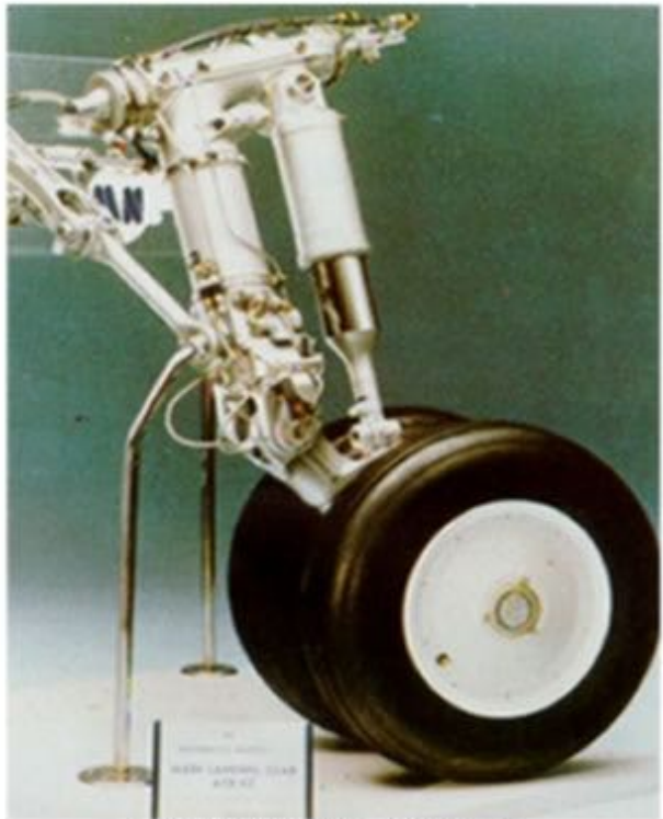
ATR42 Carrello principale ATR42 Main landing gear
