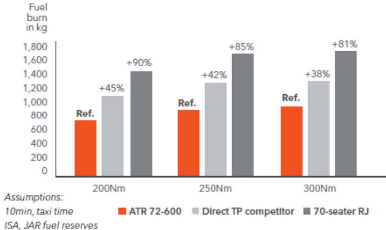
Thanks to lighter structure, optimized speed and an engine designed for short sectors, the ATR72-600 is, by far, more fuel efficient than any other 70-seater aircraft.
