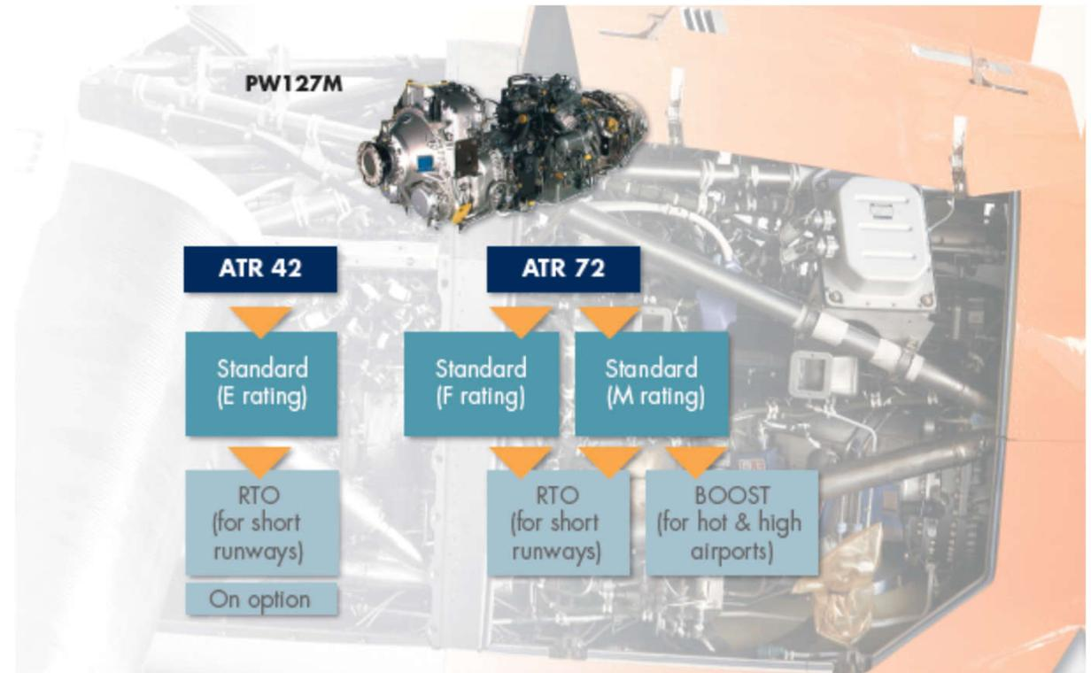
Engine rating selected through airframe identification system (EECR Electronic Engine Control Rating). Through the 'Flex Operation' concept, two levels of power are available for ATR72, allowing either PW127F ratings for standard operations or PW127M for 'Hot &High' operations
