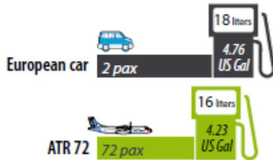
On a 200 Nm sector, the ATR 72-600 fuel consumption per passenger is up to 11% lower than a typical European car.
