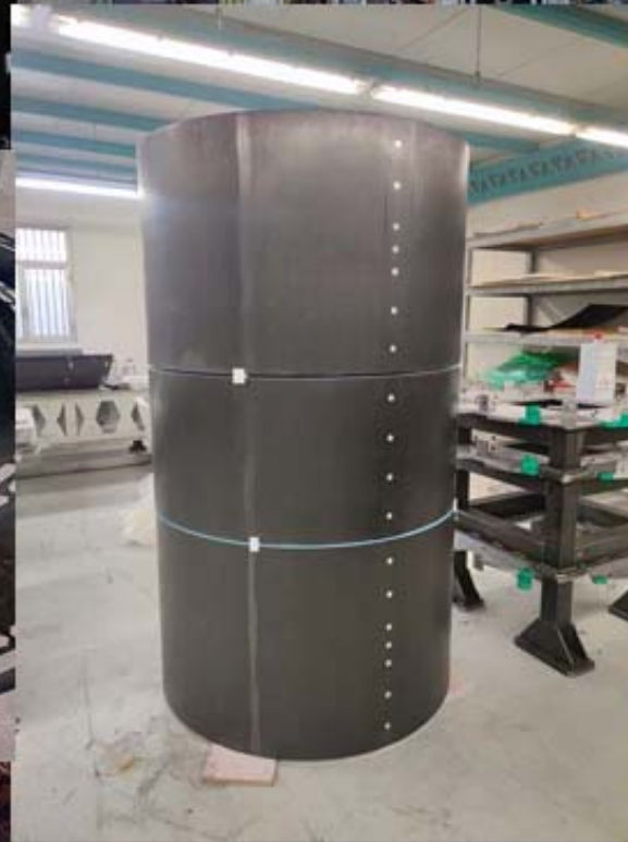
The TB2S Wheel is 2.4 m long and 2.3m in diameter
